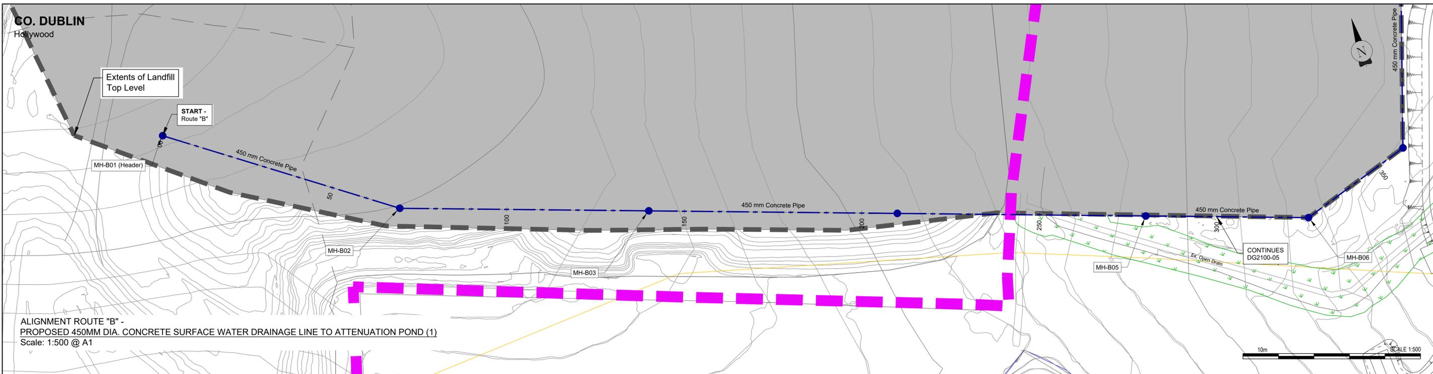
ALIGNMENT ROUTE "B" - PROPOSED 450MM DIA. CONCRETE SURFACE WATER DRAINAGE LINE TO ATTENUATION POND (1)
